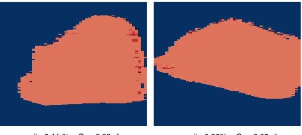
pyrite 0,11 % C<sub>Au</sub>=0,03g/t pyrite 0,85% C<sub>Au</sub>=0,05g/t Radiographic images of "hollow" stones.
