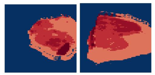
pyrite 38,63%  $C_{Au}$ = 9,18g/t pyrite 45,54%  $C_{Au}$ = 2,92g/t Images of stones from the group of large sulfides and sulfides graded by intensity.
