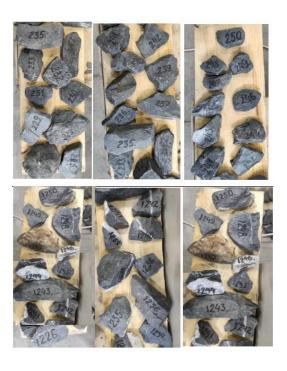
Each piece of sample was washed, labeled, weighed and sent for X-ray absorption measurements to obtain X-ray radiographs. The radiographs were processed to obtain 2 signs of separation.
