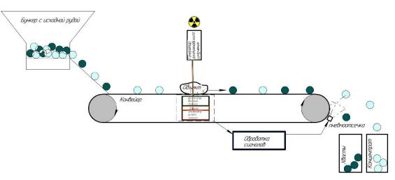
General principle of operation of the X-ray absorption sorting
